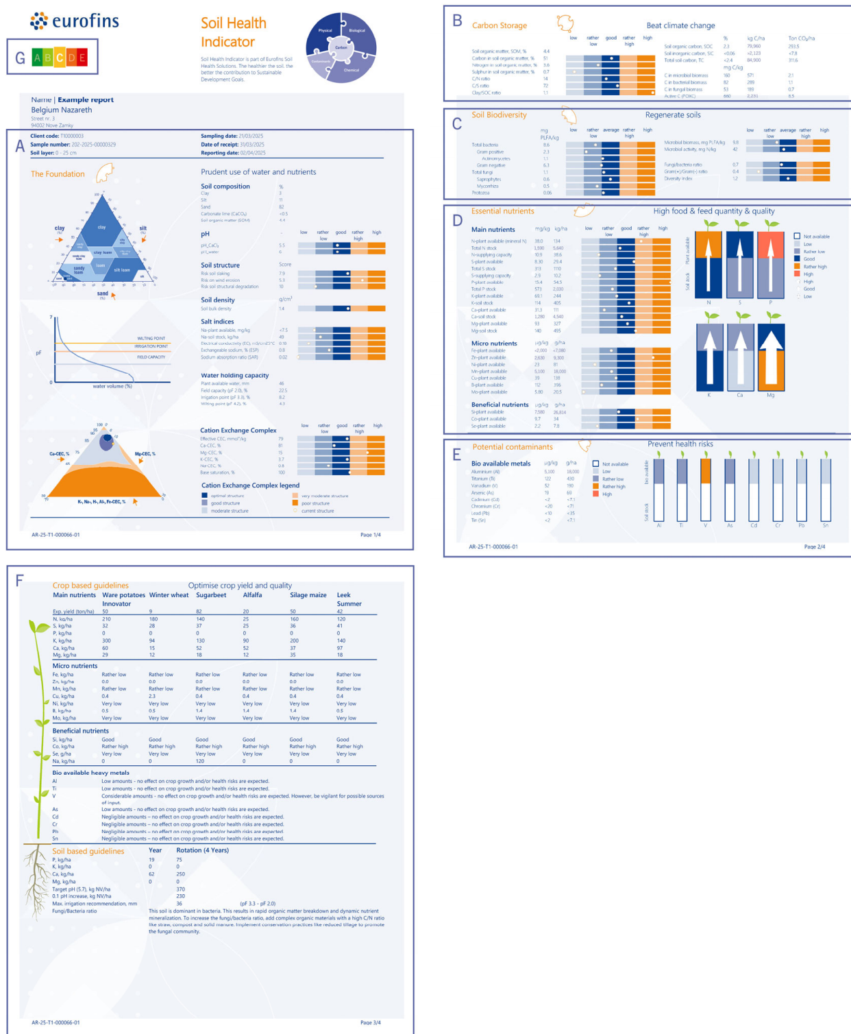
Figure 2. The soil health indicator report has 7 sections, (A) soil physical part (B) biological characteristics, (C) carbon fractions, (D) essential (chemical) elements, (E) potential contaminants, (F) crop and soil based guidelines and (G) ABCDE-score.
