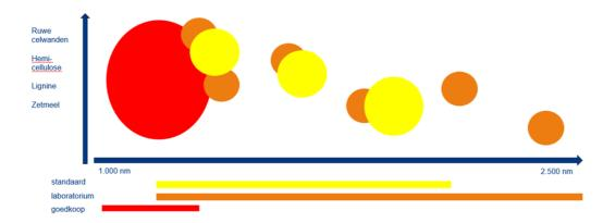
The broader the wavelength range of a NIRS device, the more detailed and accurate the analysis. Handheld scanners, like the Trinamix device(yellow) distinguish between fibre, protein, and starch. The Eurofins Agro in-lab device (orange) goes further, differentiating between fibre types and protein structures. Low-range sensors (red) can only confirm the presence of certain nutrients in feed.
